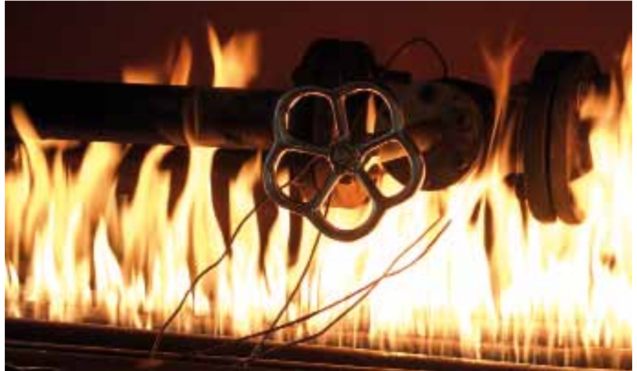
Increasingly in demand in the field of LNG: valves with Fire Safe approval
