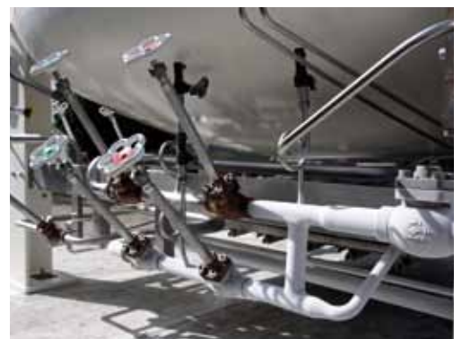
The HEROSE valves on the tank
