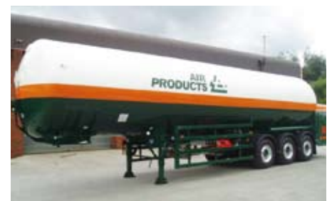
M1 CARRYMORE™ Cryogenic Road Tanker
