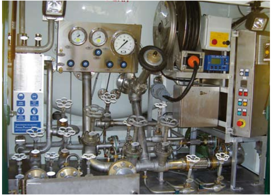
M1 Cryogenic Road Tanker control cabinet with new HEROSE gate valves. Low temperature gate valve family 09340 (on right)
